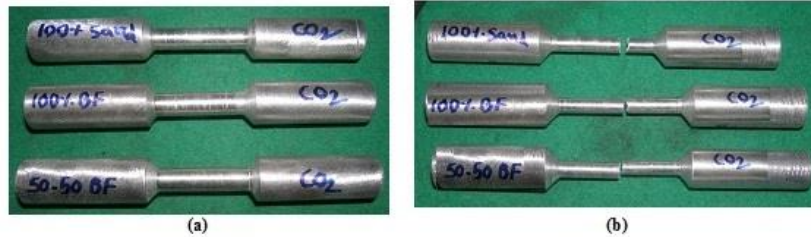
Fig. 3. Tensile specimens: (a) before testing (b) after testing
