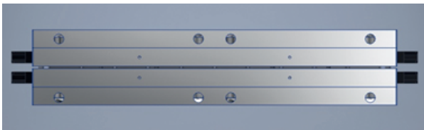
Fig. 1. Heat exchanger for liquid-liquid thermoelectric modules: a) 3D model of thermoelectric heat exchanger and its implementation (b)
