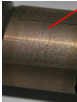
Fig. 8. Camshaft of the 126A1 engine and its elements: a) 1 and 2 – main spigots; 3 and 4 – cams, 5 – gear of the drive the ignition device; b) spigot after laser ablation texturing – bowl-shaped micro-containers, magn. 12x [4]
