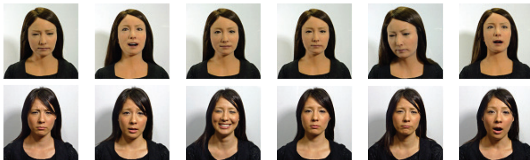
Figure 5. The android robot Geminoid F (top row) and its model person (bottom row) portraying five basic emotions and a neutral expression, from left to right: angry, fearful, happy, neutral, sad, surprised
