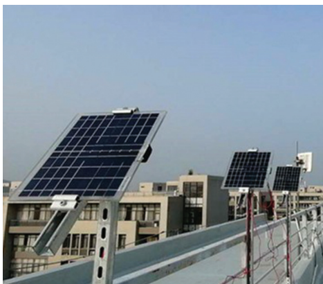
Fig. 17. bPV array optimal spacing test. bPV, bifacial photovoltaic.
