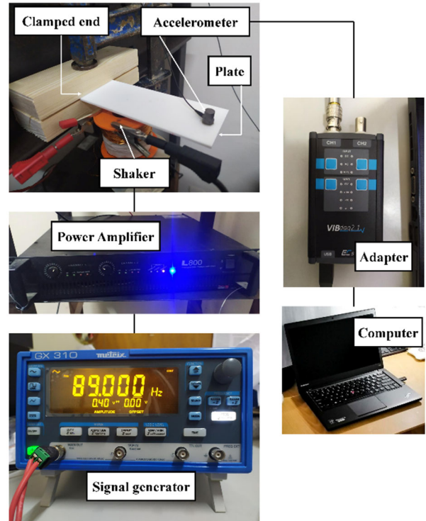
Fig. 3. Test rig for determining the dynamic characteristics for cantilever plate
