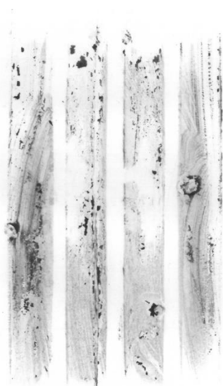
Fig. 2. Negative tire-surface contact area for the T520 tire
