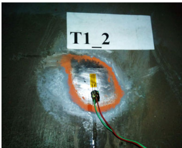
Fig. 5. Strain sensor T1_2 attached to the web of the beam 1
