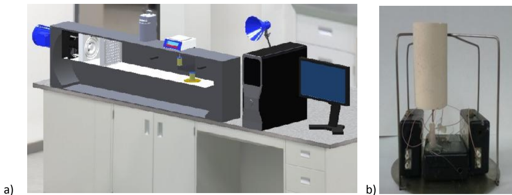
Fig. 2. View of the drying tunnel (a) and sample on weighing dish with temperature and pressure sensor (b)
