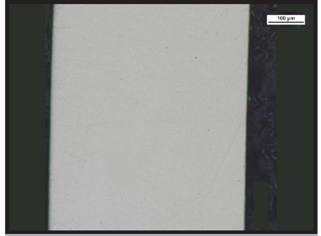
FIG. 2. Metallographic section of Adenta orthodontic wire. Non-Etched state. LM
