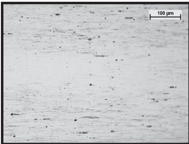
FIG. 3. The microstructure of the G&H Orthodontics orthodontic wire. Visible fibrous texture and precipitations of the Cr 23 C 6 carbide arranged in bands. Etched state. LM
