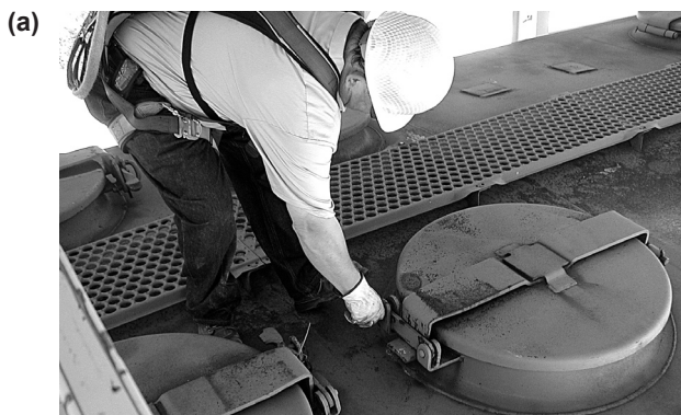
Figure 6. Rail cover latch released (a) manually and (b) with a hand tool.
