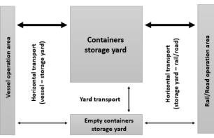
Fig. 2 Flow direction of containers in marine intermodal terminals
