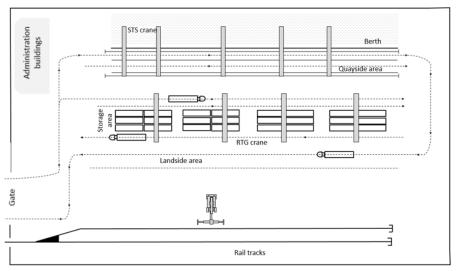
Fig 4. Marine intermodal terminal example
