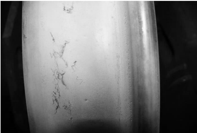
Fig. 1. Visual attributes of metal fatigue on rolling surface of wheel
