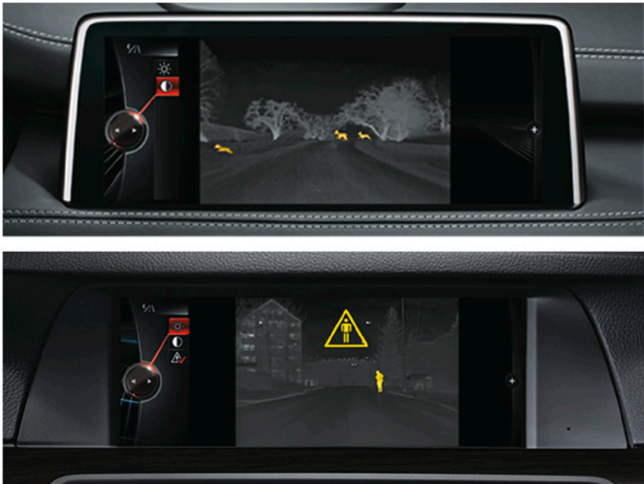
Fig. 9. Example of signalling the recognition of animals and humans by night vision systems in BMW vehicles (source: www.bmw.pl )
