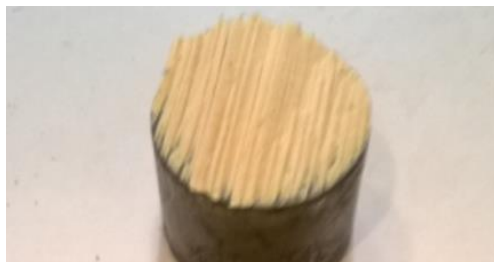
Fig. 6. Failed timber-adhesive joint after pull-off testing of Sika®PS polymer
