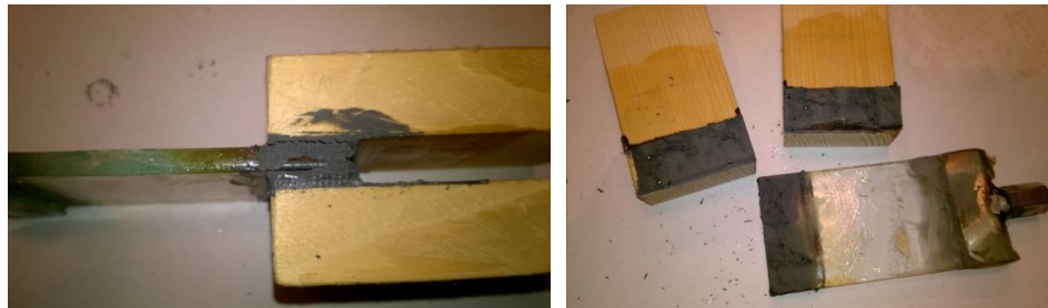
Fig. 10. Failed double lap joint (left), morphology of slide plane in adhesive layer (right)
