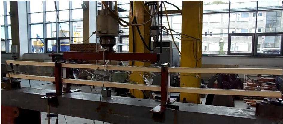
Fig. 16. Photo of failed composite timber-glass I-beam
