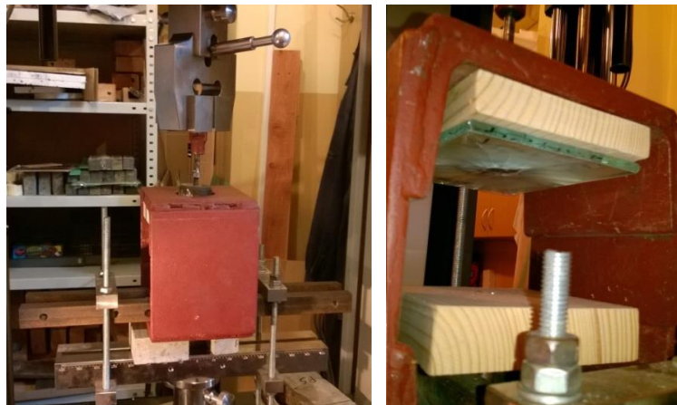
Fig. 5. Timber element (left) and glass element with timber spacer (right) mounted in the investigation tool during the pull-off tests
