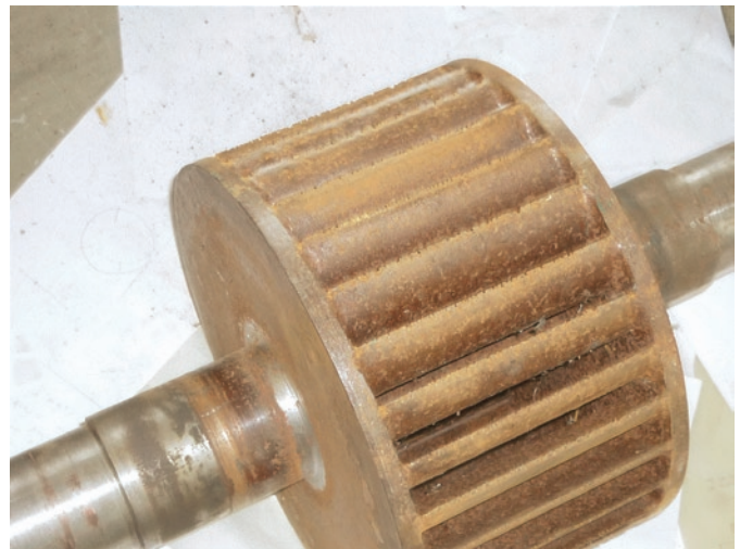
Fig. 1. Banki-Michel turbine employed for investigations. Maximum prospective power of the turbine was 13 kW
