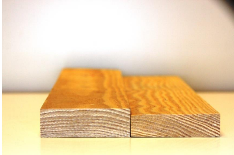
Fig. 1. Samples of Scots pine ( Pinus sylvestris L. ) and thermomechanically densified Scots pine.
