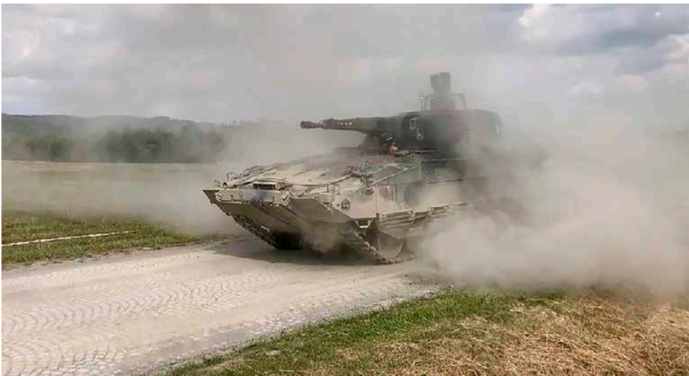
Fig. 9. A Puma infantry fighting vehicle which utilises a solution involving low placement of the exhaust system and dispersion of the heated exhaust fumes towards the ground
