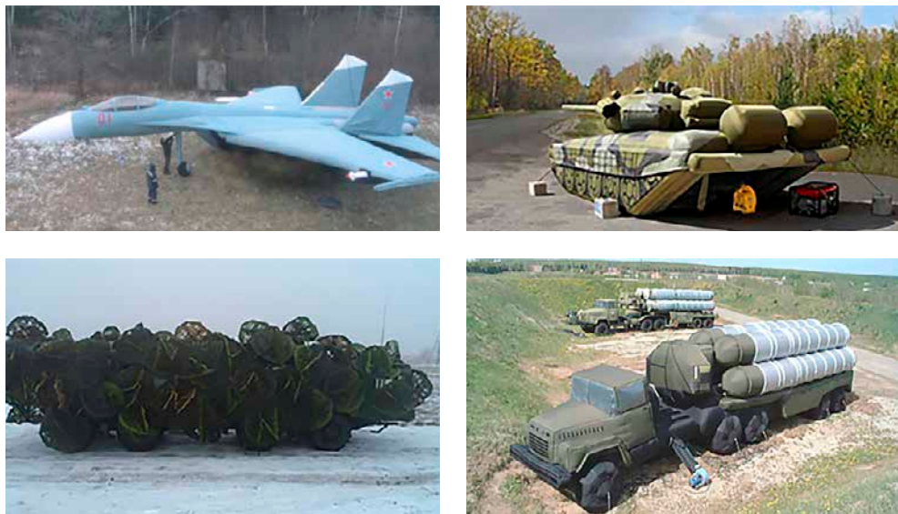
Fig. 7. Mock-ups of an aircraft, a tank, a rocket launcher and a camouflaged anti-aircraft system at the disposal of the camouflage subunits of the Russian Armed Forces Source: [19].
