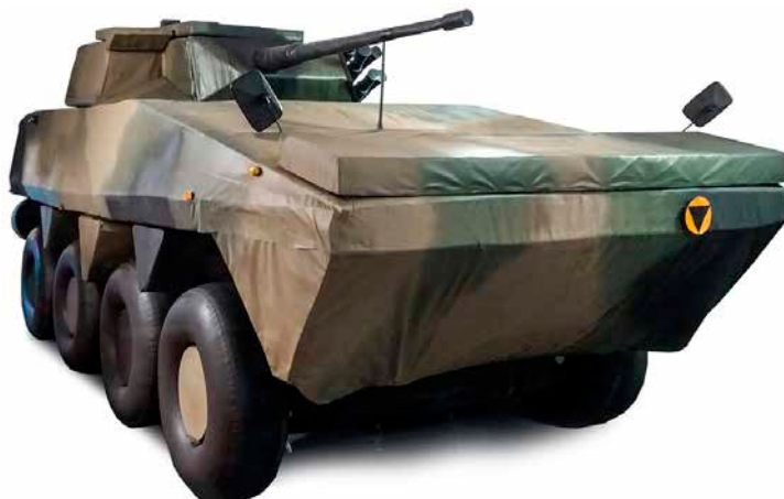
Fig. 3. Pneumatic mock-up of a ROSOMAK wheeled armored personnel carrier Source: Lubawa S.A. information materials.
