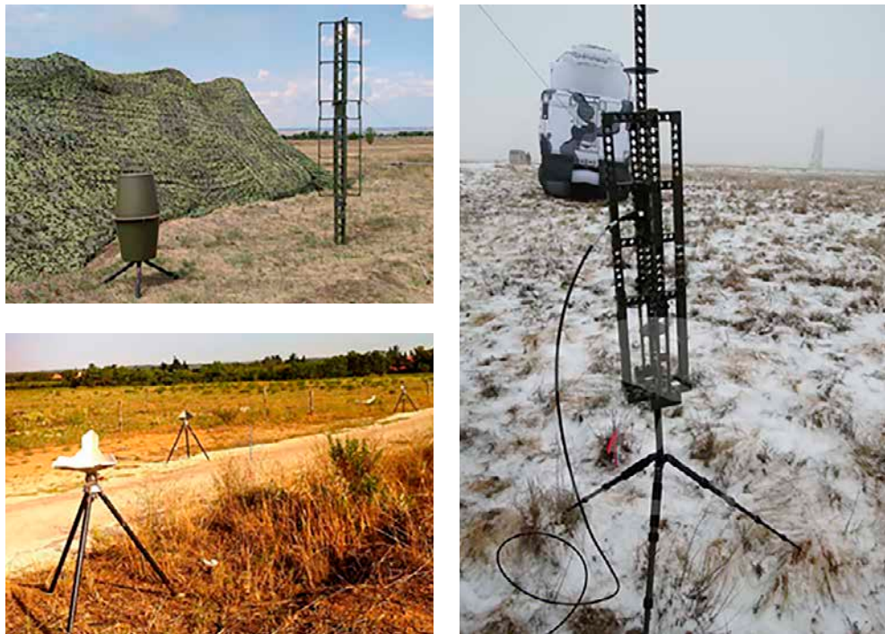
Fig. 8. Electronic dummy objects combined with 3D mock-ups and corner reflectors allow for a more realistic simulation of command systems at the tactical level Source: [20].
