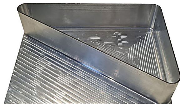
Fig. 6. Tested thin-walled structure
