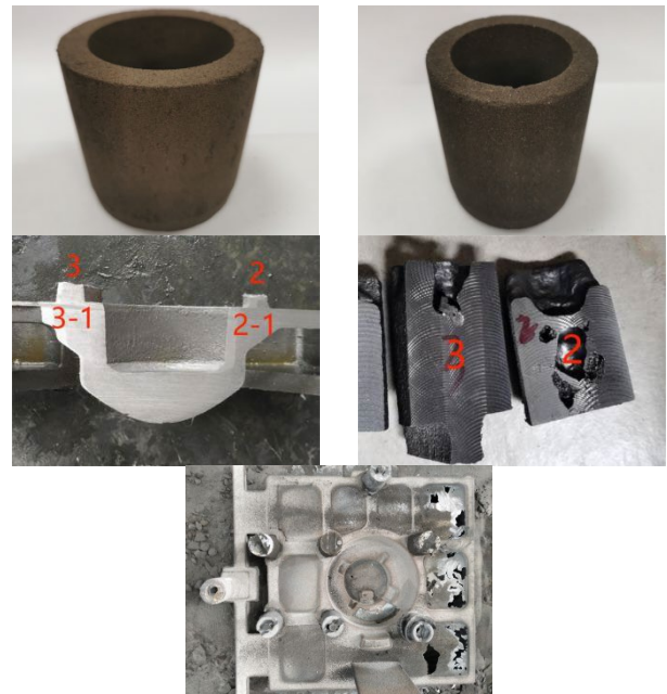
Fig.5. Casting experiment: a) Arc flue ash riser sleeve, b) Iron black riser sleeve, c) casting profile, d) riser sleeve inner profile, e) wheel casting
