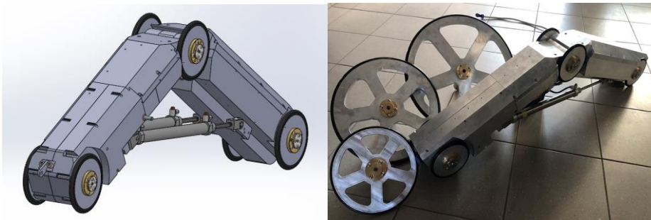
Fig. 1. 3D and physical models of the propulsion module
