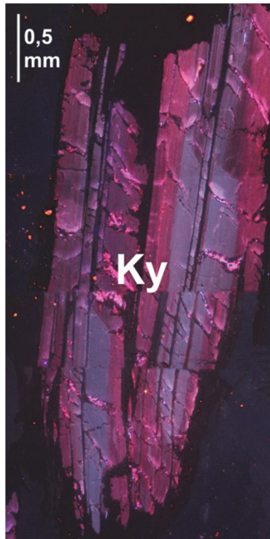
Fig. 7. Cathodoluminescence image of kyanite crystal.
