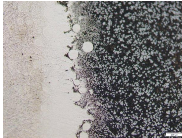
Fig. 3. Microstructure of the fusion border, pad-weld – left side, substrate – right side
