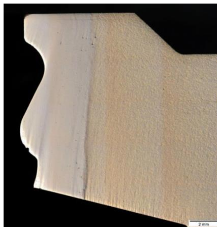
Fig. 2. Cross-section of the pad-weld along the radius of the form, image without etching
