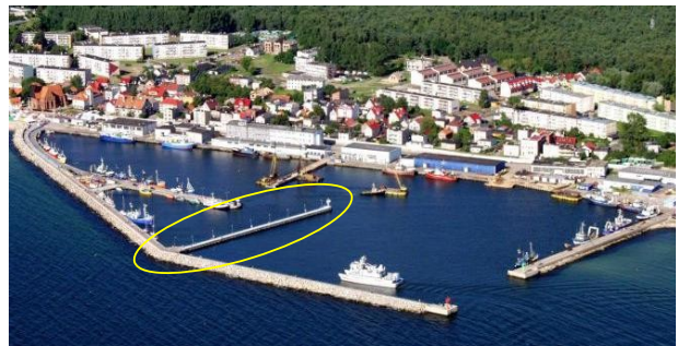
Fig. 10. The fishery harbour in Hel. The designed fish pier is marked yellow [ http://www.maszwojne.pl ]
