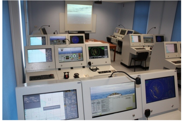
Fig. 8. Integrated simulator RADAR-ARPA/ECDIS-WECDIS [archives of INiHM]
