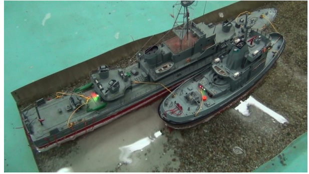
Fig. 2. Washing out sea bottom by a rescue ship before re-floating the vessel [archives of Department of Ship's Operation]
