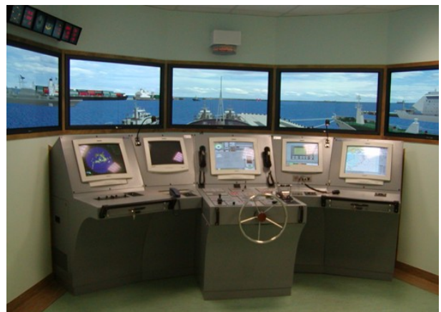
Fig. 4. Integrated multitask simulator of the navigational bridge [archives of INiHM]
