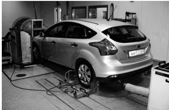
Fig. 2. Exhaust emissions laboratory at BOSMAL, showing the chassis dynamometer, windspeed fan and a vehicle, all within the climatic chamber
