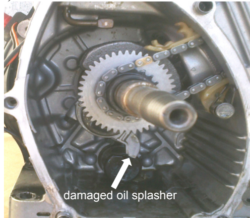
Fig. 2. Damaged oil splasher (a) and location of the air filter (b)
