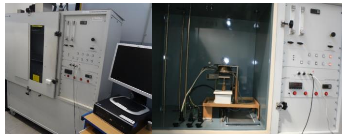
Fig. 14. Test stand according to PN-EN ISO 5659-2 (source: Railway Institute)
