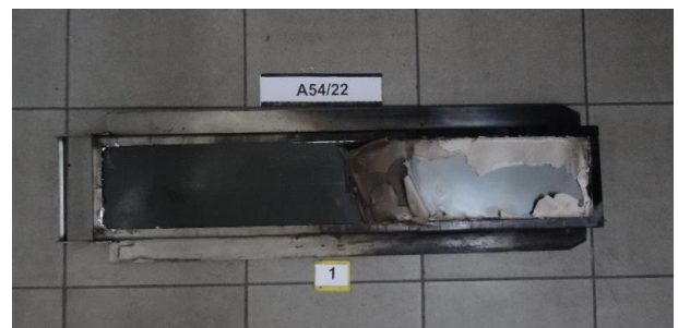
Fig. 5. A sample of the painting system after the test
