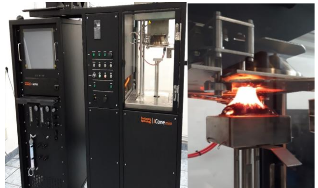
Fig. 8. Test stand according to ISO 5660-1 and a sample during the test (source: Railway Institute)
