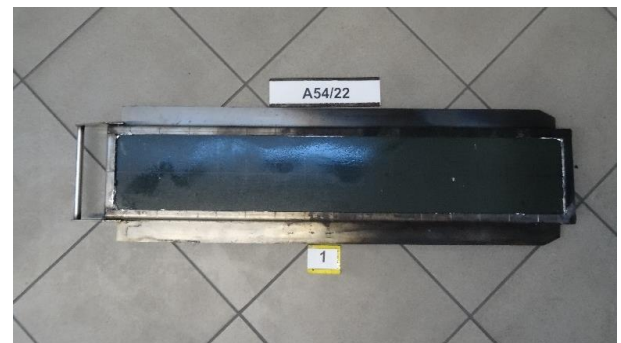
Fig. 4. Paint system sample before testing
