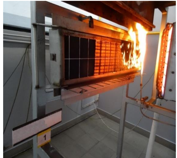
Fig. 3. Material sample during CFE determination (source: Railway Institute)
