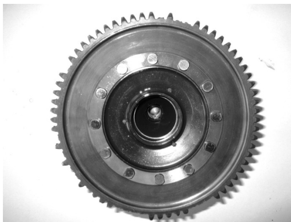
Fig. 15. Damage of gear of generator power gearbox – multiple tooth break-off is noticed
