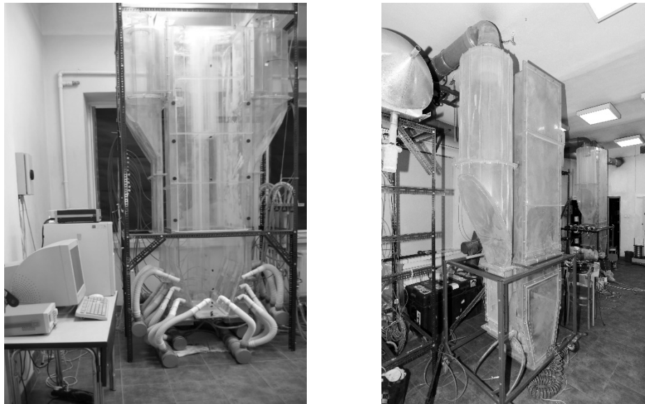
Fig. 1. Cold models of: a. Lagisza 966 MW th CFB boiler - scale 1/20, b. Fortum 120 MW th CFB boiler - scale 1/10
