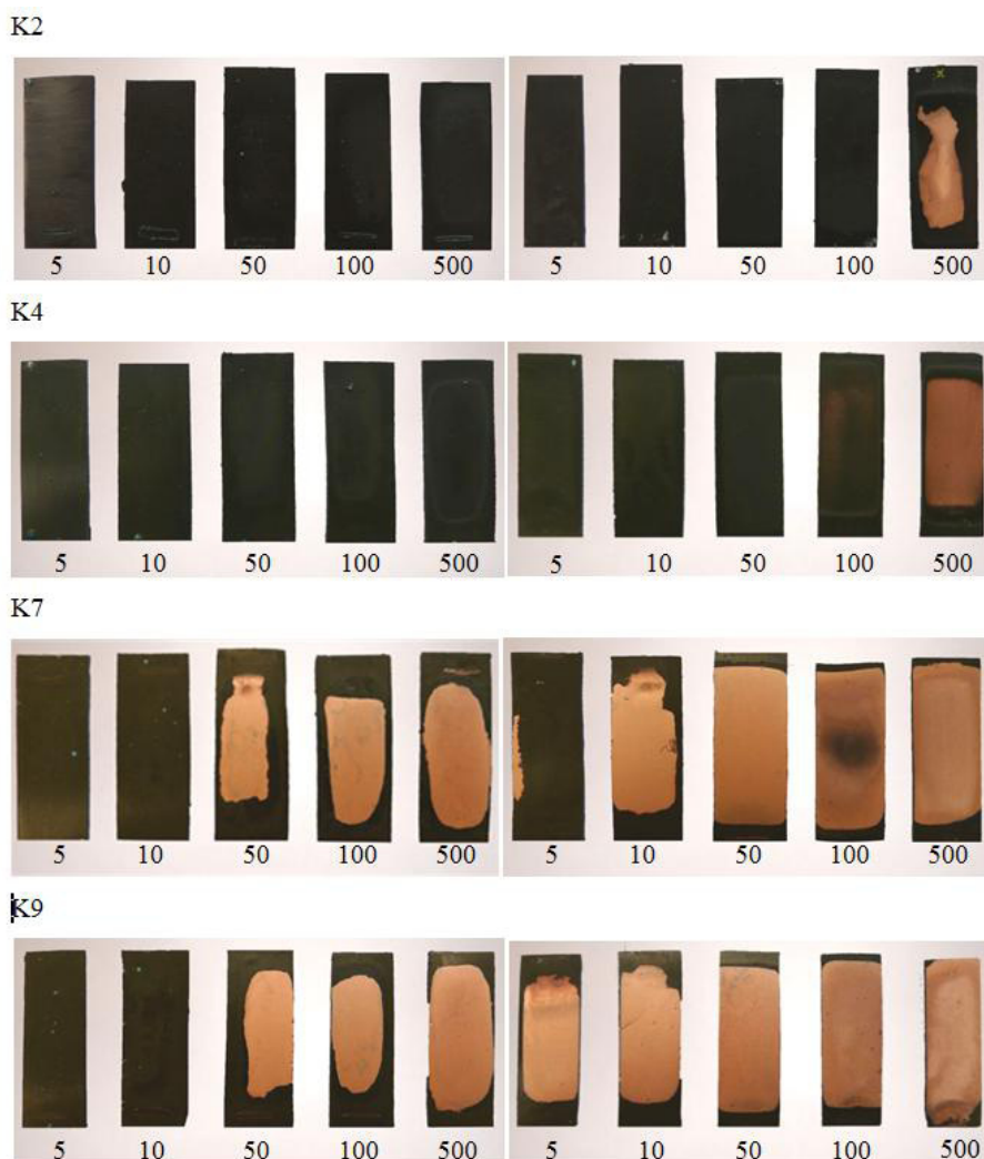
Rys. 1. Wyniki miedziowania próbek kompozytów K2, K4, K7 i K9; w każdym wypadku 5 pierwszych próbek napromieniano impulsami o E_{j1} = 40 \text{ mJ/cm}^2 , 5 kolejnych – impulsami o E_{j2} = 120 \text{ mJ/cm}^2 ; liczby pod każdą z próbek oznaczają liczbę impulsów laserowych [6] Fig. 1. Results of copper plating of K2, K4, K7 and K9 composite samples (for each series the first five samples were irradiated with laser pulses of fluence E_{j1} = 40 \text{ mJ/cm}^2 , and next 5 pulses at fluence of E_{j2} = 120 \text{ mJ/cm}^2 ; numbers below each sample indicate number of pulses) [6]
