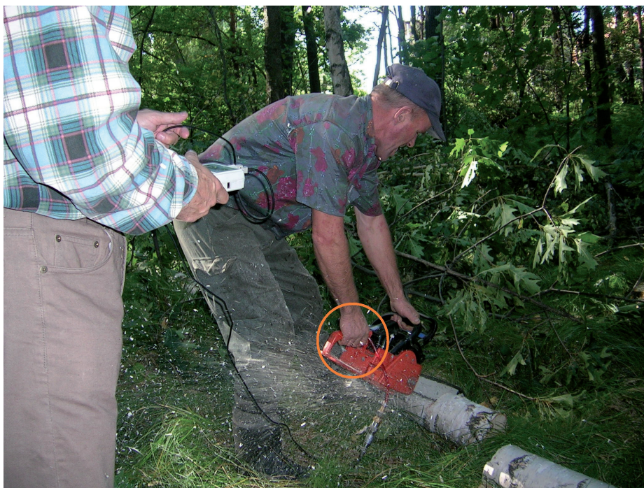
Figure 2. Measurement of coupling forces applied by a forestry worker with his right hand. Notes. The active liquid pad is circled.
