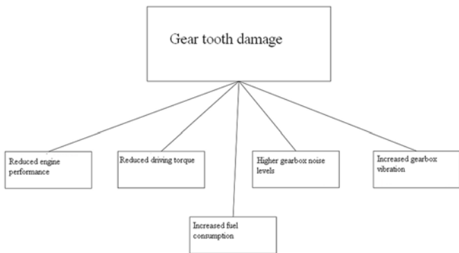
Fig. 6. Diagnostic symptoms of gear tooth damage
