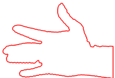
Fig. 23. Sample improper segmentation result (missing valley points).
