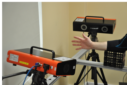
Fig. 1. 3D data acquisition station (hand scanning process).
