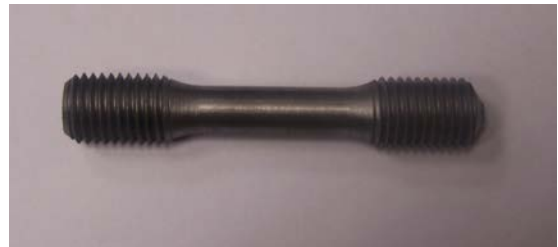
Fig. 3. A specimen for mechanical testing made of material cut out of a collar of a casting
