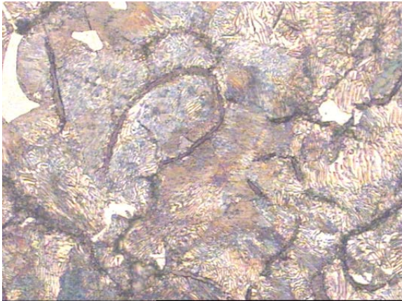
Fig. 5. Microstructure of cast iron inoculated with Zircinoc master alloy; etched with Nital, magn. 400×
