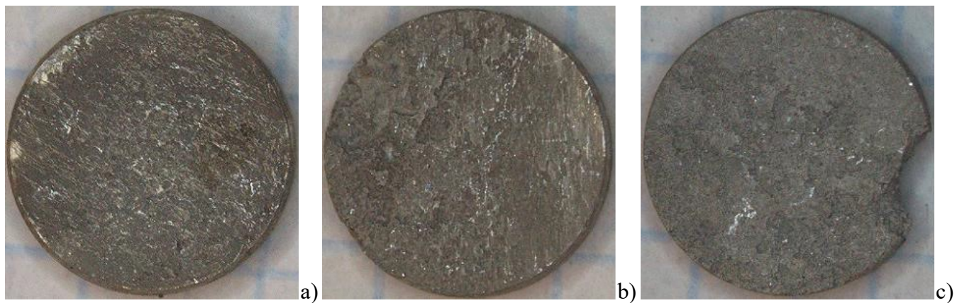
Fig. 4. Surface of samples after immersion tests performed during 6 days in NaCl solution with concentration of: a) 0.01 M, b) 0.6 M, c) 2.0 M
