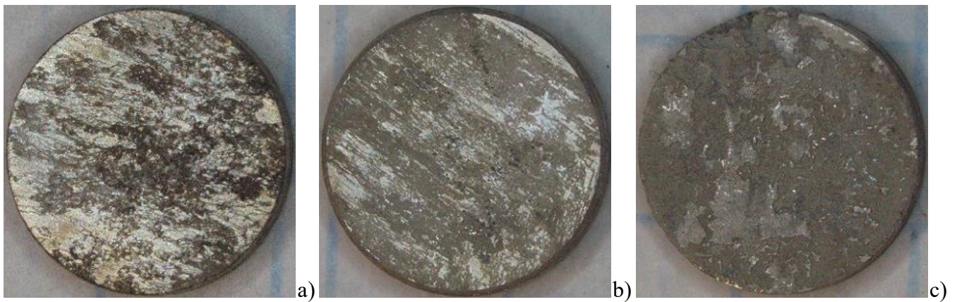
Fig. 3. Surface of samples after immersion tests performed during 3 days in NaCl solution with concentration of: a) 0.01 M, b) 0.6 M, c) 2.0 M
