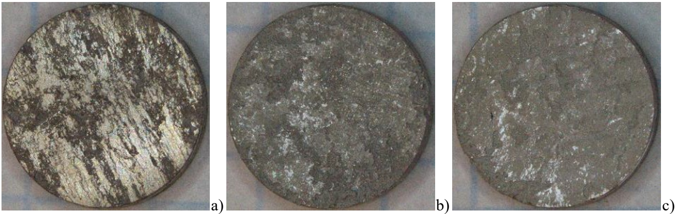
Fig. 2. Surface of samples after immersion tests performed during 24 h in NaCl solution with concentration of: a) 0.01 M, b) 0.6 M, c) 2.0 M
