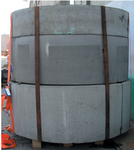
Fig. 8. Concrete manhole during testing
