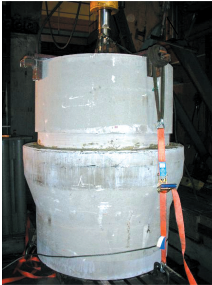
Fig. 6. DN 1000 reinforced concrete socket pipe joint in the test facility
