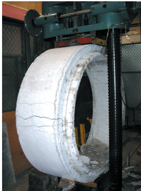
Fig. 12. 1500 mm diameter reinforced concrete ring during the crushing test
