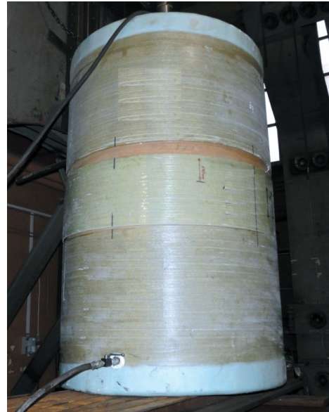
Fig. 7. DN 1300 GRP casing pipe joint in the test facility
