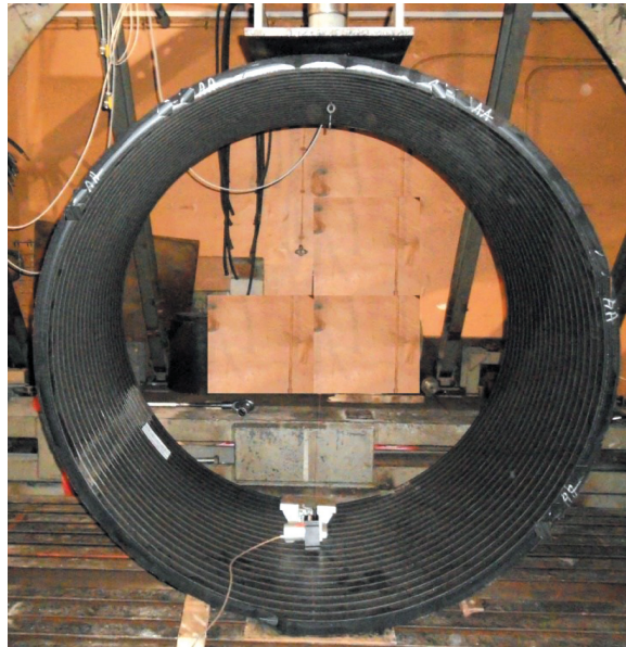
Fig. 11. DN 1500 pipe in the test facility
