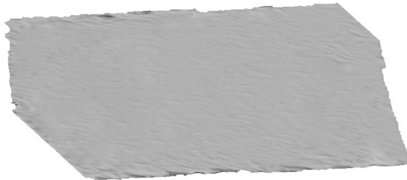
Fig. 9. Top view of the reconstructed plane using the data extracted from the images and homographic techniques after the correction of the refraction deformation.
