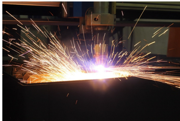
Fig. 11 Material spattered during penetration
