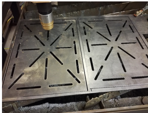
Fig. 10 Burnouts with visible exits outside the contour (at the bottom edge of the material)
