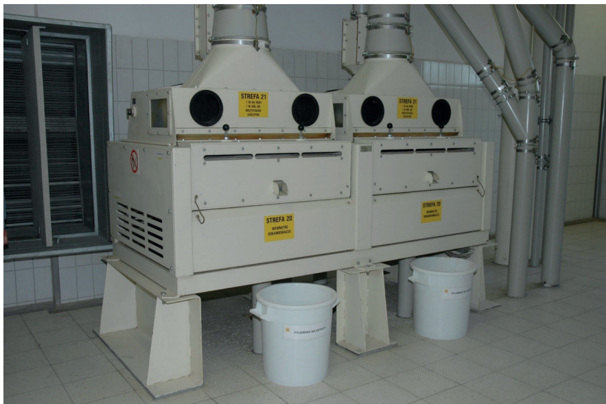
Fig. 10. A set of sieves resting on the floor slab in the production building of the industrial plant – the object is not the structure
