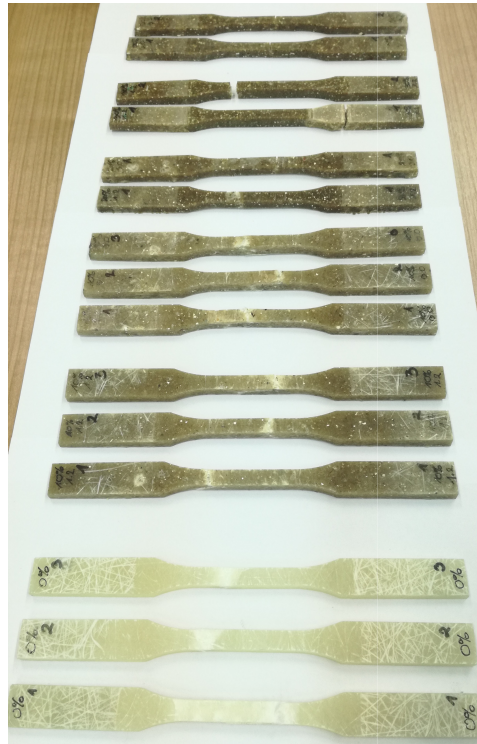
Fig. 3. Samples after static tensile testing
