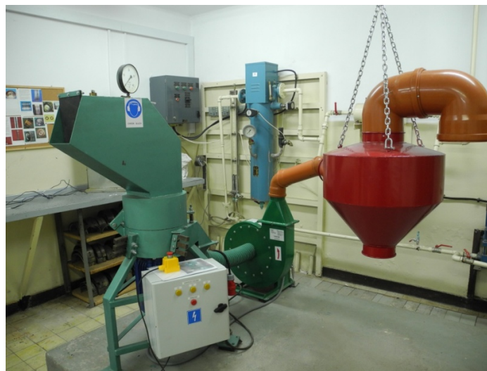
Fig. 1. Crusher – a processing station for composite materials [7]
