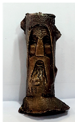
Fig. 2. Picture of the obtained complex relief MMC with copper alloy (CuZn38Pb2) matrix and Fe reinforcing phase
