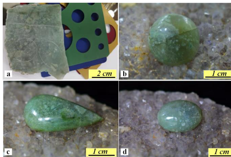
Fig. 8. Cut plates from Ch-chalcedony (a), circle (b), drops (c), and oval (d) forms in the cabochon cutting
