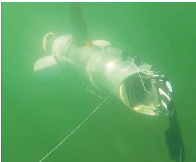
Fig. 2. BUV with two side fins and one flexible tail fin [15]
