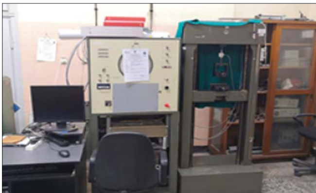
Fig. 7. Laboratory station for measuring Young’s modulus
