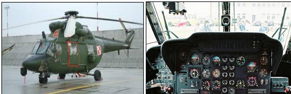
Fig. 6. View of the W-3WA Sokół helicopter with analogue on-board systems (left) and the panel of instruments with analogue avionics elements (right)
