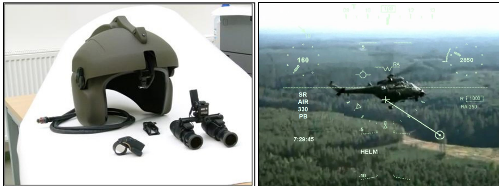
Fig. 7. View of the WDN-1 helmet-mounted display installed on the THL-6NSC/P pilot's helmet (left) and imaging the piloting-navigational and targeting parameters (right)
