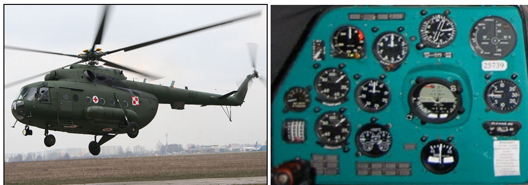
Fig. 1. View of the Mi-17-1V helicopter with the SWPL-1 Cyklop digital system (left) and the current panel of analogue on-board instruments (right)
