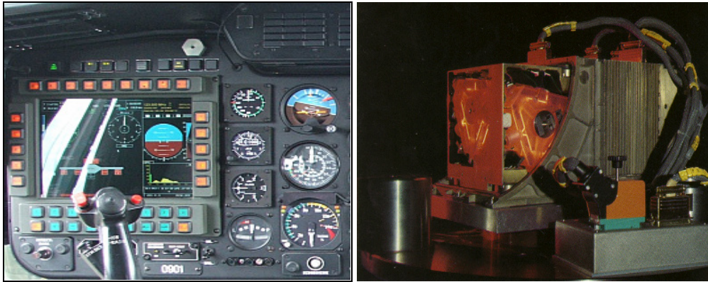
Fig. 8. View of imaging the piloting-navigational parameters on the MW-1 multifunction monitor screen (left) and the EGI-3000 inertial navigation unit providing these parameters (right)
