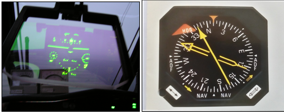
Fig. 9. View of imaging flight parameters on the HUD transparent indicator (left) and imaging the heading on the KNI-582 radio magnetic indicator (right)
