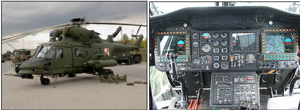
Fig. 5. View of the W-3PL Głuszczyk helicopter with the integrated avionics system (left) and the panel of instruments with digital avionics elements (right)
