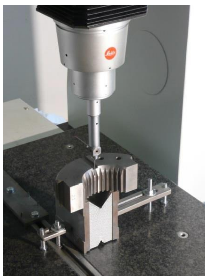
Fig. 7. An idea of coordinate metrology.
