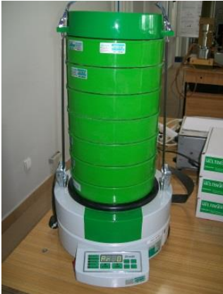
Fig. 6. Place of the determination of granules equivalent diameter
