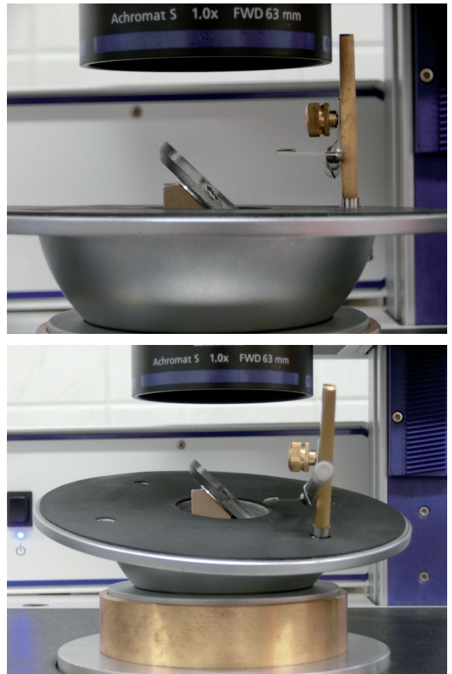
Figure 3 Tilting stage with a handle and built-in flat mirror in selected positions
