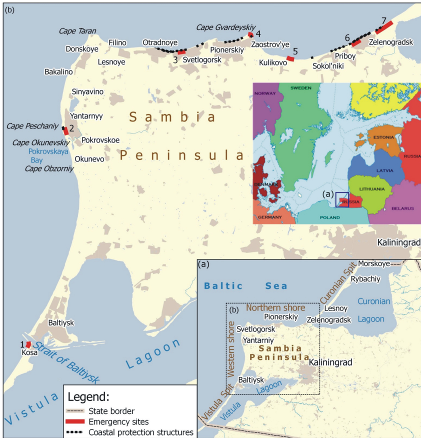
Fig. 1. Kaliningrad Oblast coastline with four major morpholithodynamic segments (a): the Russian part of the Vistula and Curonian spits, the western and northern shores of the Sambia Peninsula. The location of emergency sites (Table 1) and coastal segments protected by engineering structures are marked in panel (b), see legend
