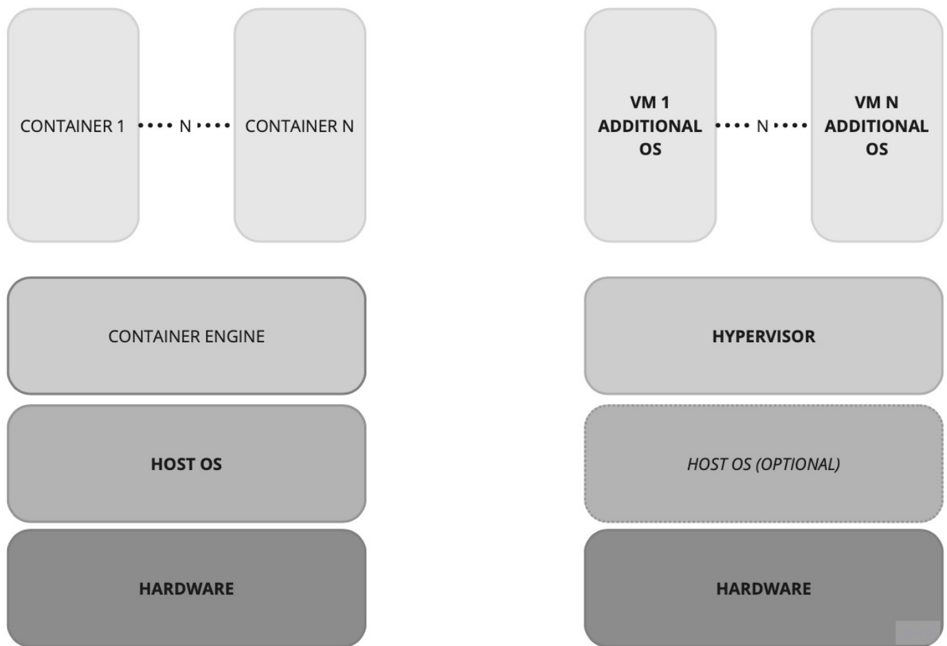
Figure 1: Architecture overview of containerization (left side) and virtualization (right side)
