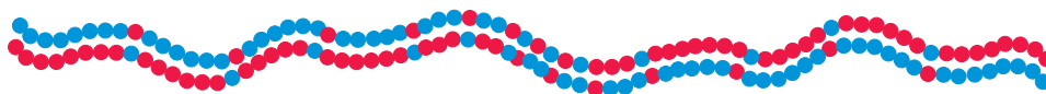
Scheme G. The structure of stereocomplex formed by block/gradient macromolecules containing long enough consecutive units of (S,S)-LA and of (R,R)-LA for stable interactions, required for stereocomplex formation
